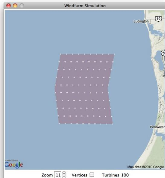
To generate the Google Earth model, the program substitutes the latitude and longitude of each turbine into an XML template, along with the bearing corresponding to the prevailing wind direction. The result is a single KML file describing the entire wind farm. To this is added the Sketchup model(s) for the turbines, and the resulting files archived as a zip (KMZ) file (the typical distribution format for a Google Earth model).
