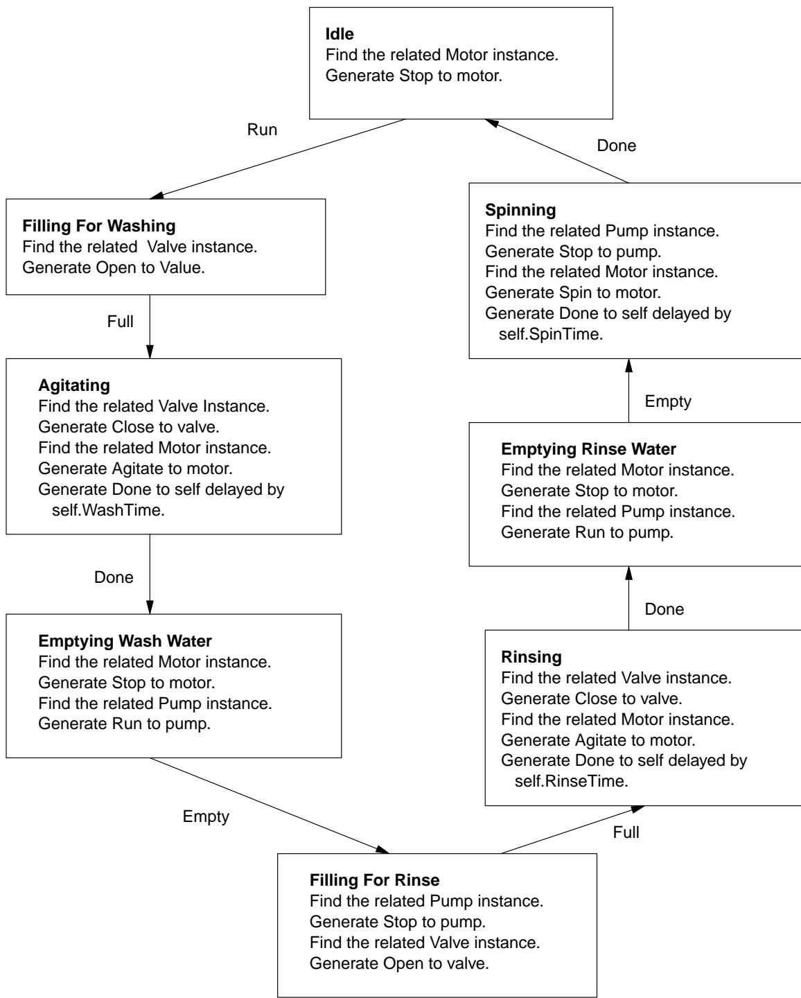
**Figure 2. State Model for Washing Machine Class**
