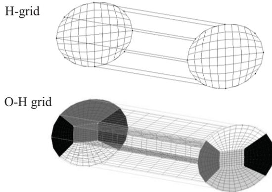
**Fig. 1 H-grid and 5 block O-H grid**
